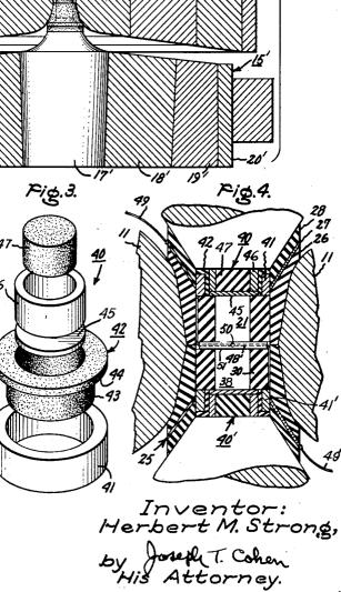
May 7, 1963 TWO-TERMINAL END CAP FOR HIGH PRESSURE, HIGH TEMPERATURE REACTION VESSELS Filed Aug. 2, 1961
