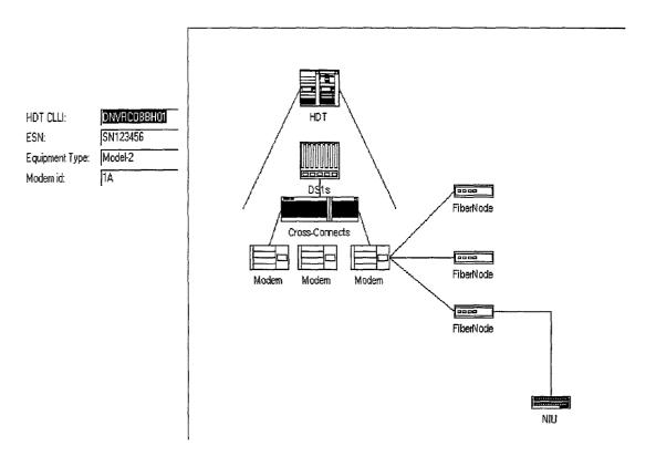
Figure 7 – Object Discovery message arriving from HDT upon the event that an NAU was powered up on the CATV network.
