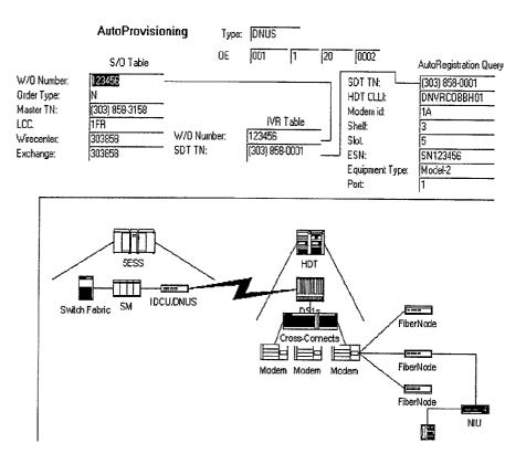
Figure 11 – The information used to establish to in-band communications channel is now correlated to the original Work Order that was entered.
