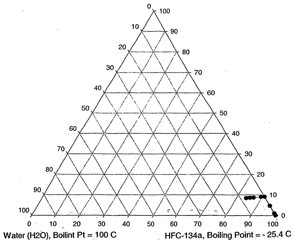
—●— Boiling Pt @ 14.57 psia along the line is within -25.4 C to -25.8 C
