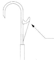
Line guide is used to keep fishing line clear of running gear and outboard motors while landing the fish
