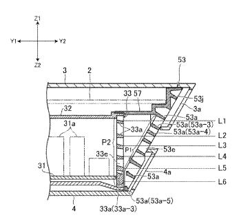
component disposed inside the electronic apparatus and the plurality of first louvers and are lined in the second direction when the vent is viewed along the first direction. A straight line that passes between adjacent two first louvers and is along the first direction intersects any of the plurality of second louvers.
