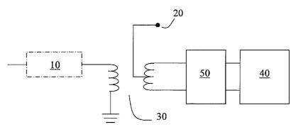
(57) Abstract: Device for reducing noise in a radio receiver, which radio receiver comprises a transformer (30) having a reference voltage input (20), a radio signal input at a first transformer side, and a radio signal output at a second transformer side, an A/D converter (40) being connected to said second transformer side, wherein a first bandpass filter (50) is connected between said second transformer side and said A/D converter.
