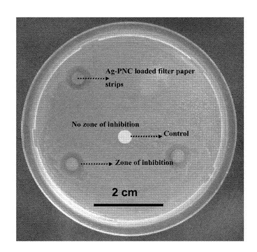
Average zone of inhibition width ~ 2.5 mm
