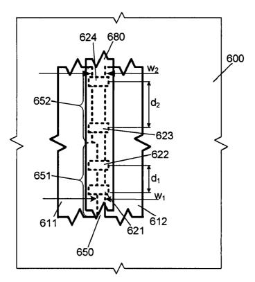
Z<sub>e</sub> = an effective impedance of a tank circuit modeling a section of gap 650,
