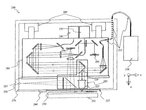
(57) Abstract: An optical inspection tool including a movable optics system is characterized in terms of position and wavelength dependent quantities over a range of motion. Once the position-dependent quantities are determined at various wavelengths and positions, they are stored and used to interpret data from test wafers having an unknown metrology. A portion of the characterization of the optical system may be accomplished by using titled black glass to provide a non-reflective reference.
