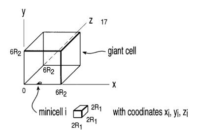
$n = 6R_2 \div 2R_1 = number of mini cells along each axis$  $n^3$  = number of minicells in a giant cell let m be number of frequency channels  $K = n^3 \div n$  = number of time slots
