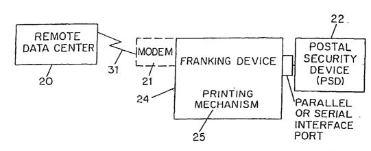
(57) Abstract: A system for printing postal indicia. The system includes at least one postal security device (22) which is linked to a customer host (24); where both the security device (22) and customer host (24) are connected to a data center (20).
