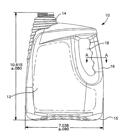
(57) Abstract: Α plastic container having a body portion and a handle portion which extends from the body portion is formed using a pair of mold halves placed into engagement. During the molding process, a surface of the handle portion is provided with a recess in at least one area where the mold halves are in placed into engagement.
