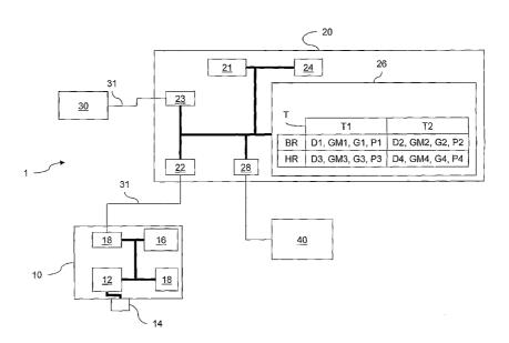
(57) Abstract: The invention relates to a system for acquiring dental radiology images, said system comprising an X-ray generator and a module for controlling an intraoral sensor. Said module comprises means for sending a control command to the generator, according to at least one pre-determined criterion, in order to prohibit, stop or modify the power of the X-ray emission. The invention also relates to the use of said system for optimising the quantity of X-rays received by a patient.
