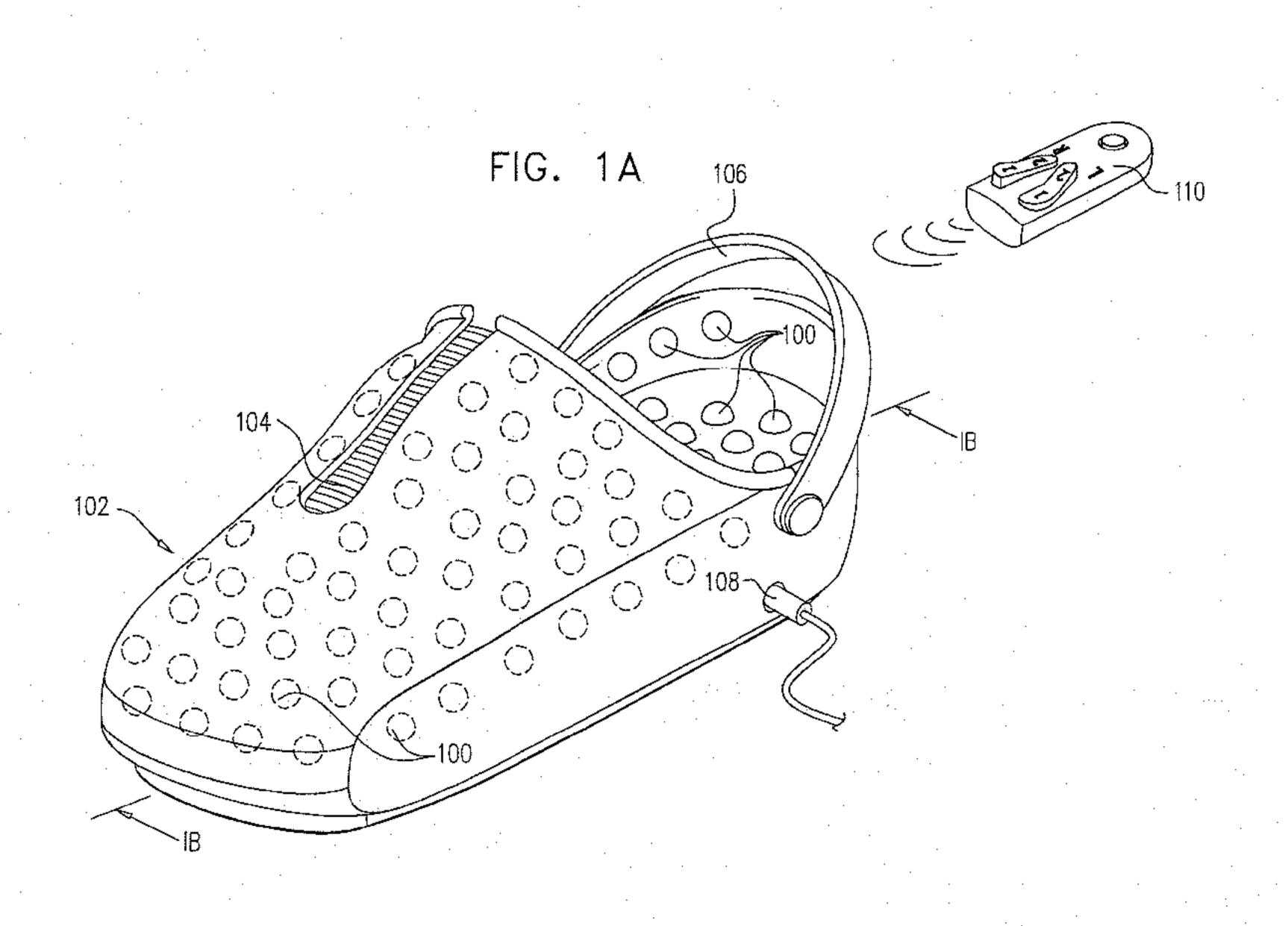
(57) Abstract: A massaging shoe including a shoe body portion formed of a vibration transmitting material and having an interior surface which includes a multiplicity of integrally formed raised surface elements and a vibrator operative to generate vibrations, the vibrations being transmitted via the vibration transmitting material and the integrally formed raised surface elements to a foot of a wearer of the shoe.
