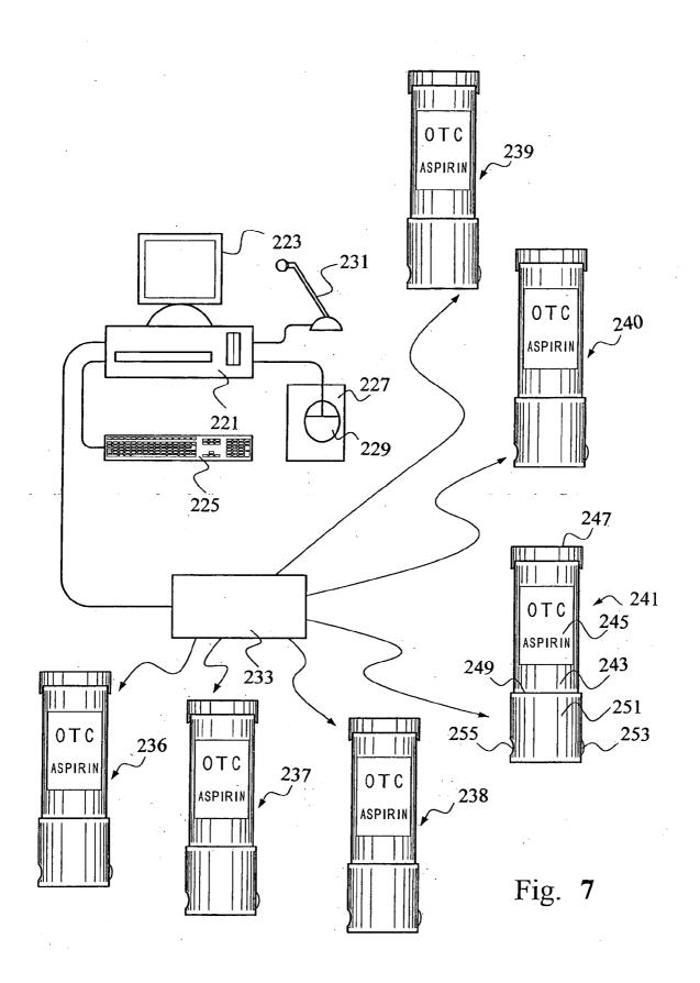
CENTRAL PROCESSOR WITH USER INPUT MEANS, WAVE FILE MEANS TO CREATE WAVE FILES DIRECTLY FROM INPUT, OR THROUGH TEXT-TO-SPEECH CONVERSION, AND WIRELESS TRANSMISSION MEANS.
