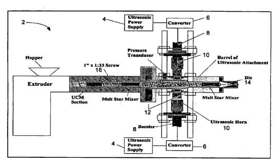
(57) **Abstract:** The present invention relates to processes for producing high performance polymer composites via ultrasonic treatment after initial mixing. These high performance polymer composites made from a combination of polymer and nanofibers and/or nanotubes. The ultrasonic treating method of the disclosed allows a more highly dispersed polymer composite mixture which provides increased thermal, mechanical and electrical properties.
