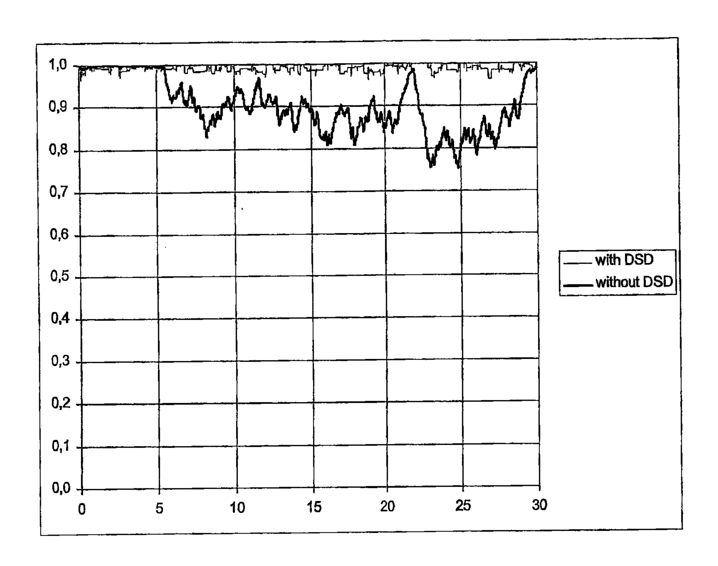
Omni parameter with and without DSD circuit
