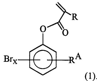
In formula 1, R can be hydrogen (-H) or methyl (-CH<sub>3</sub>), R<sup>A</sup> can be a straight or branched alkyl preferably having from 1 to 18 carbon atoms, and x can be in the range from about 1 to 4, with the combination of these variables preferably being 10 such that the brominated monomer has an index of refraction of at least 1.50. R<sup>A</sup> can be positioned ortho, meta, or para to the ester.
