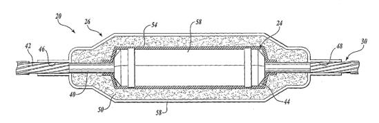
(57) Abstract: Embodiments of a fluid storage and introduction device (20) constructed in accordance with respects of the present invention are provided. One embodiment of the device (20) includes an inner assembly (24) and an outer housing (26). When assembled, the device (20) is securely coupled to a cable or cable section (30) along a portion of its span. In use, the device (20) is capable of storing remediation fluid and introducing such fluid into the cable or cable section (30).
