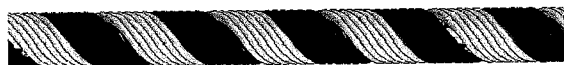
Series of ribbon cables can be coiled together to form multi-conductor lead
