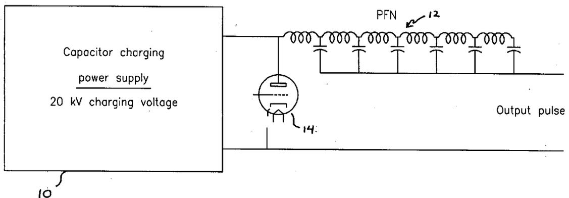
Modulator with Capacitor Charging Power Supply
