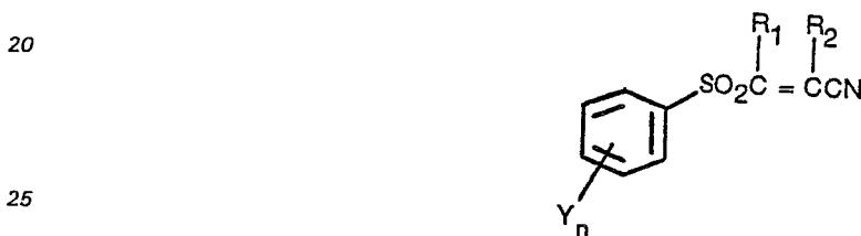
in which Y is hydrogen, halogen, C<sub>1</sub>—C<sub>4</sub> alkoxy, or C<sub>1</sub>—C<sub>4</sub> alkyl; R<sub>1</sub> and R<sub>2</sub> are independently hydrogen or methyl; and n is 1 or 2, in an amount of 12 to 13% by weight and an extrusion aid.
