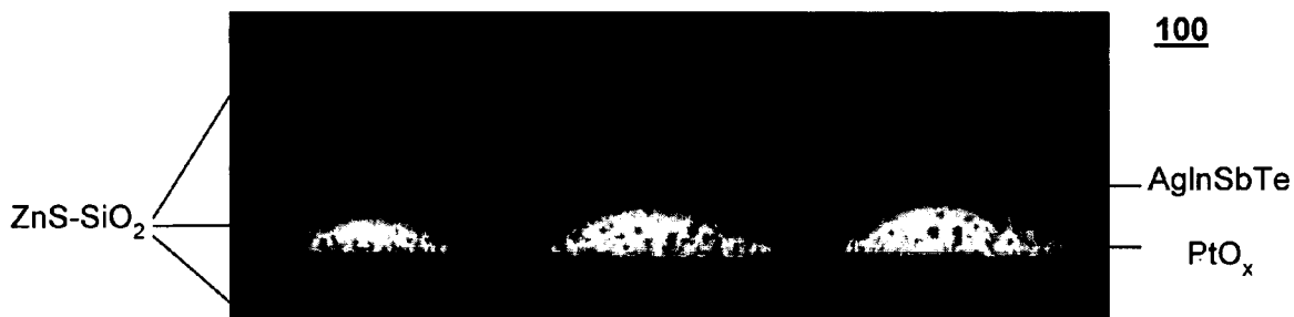
Super resolution optical disc transmission electron micrograph
