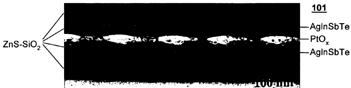
Super resolution optical disc transmission electron micrograph
