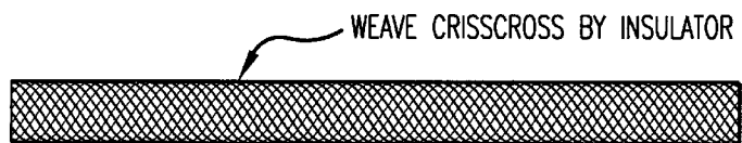
A EXAMPLE OF A PARALLEL CONDUCTOR
