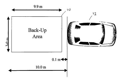
(57) Abstract: A back-up aid indication system includes a sensor for providing detection coverage in a predetermined coverage zone behind a vehicle. The sensor includes a transmit antenna adapted for transmitting an RF signal having a quasi-collimated antenna pattern in a near field. The system further includes a waveform generator which selectively provides one of a frequency modulated continuous wave FMCW Chirp signal and a pulse waveform signal as the transmitted RF signal.
