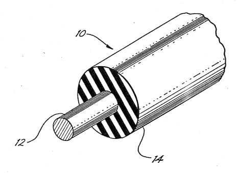
FLAME-RESISTANT HYDROCARBON POLYMER COMPOUNDS, AND INSULATED ELECTRICAL PRODUCTS THEREOF
