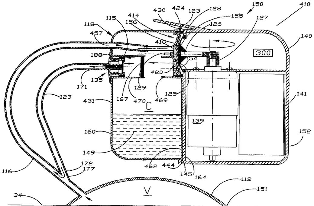
(57) **Abstract:** A suction head in fluid communication with a pump head (414) provides a sub-ambient working pressure to a target area, enabling drainage thereof to a waste container. A passive pressure regulation system (135) enables the working pressure to be maintained at a desired level. A monitoring system for a suction system is also provided.
