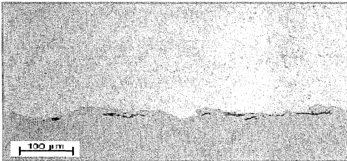
FIGURE 26 B The Cu has a flattened structure
