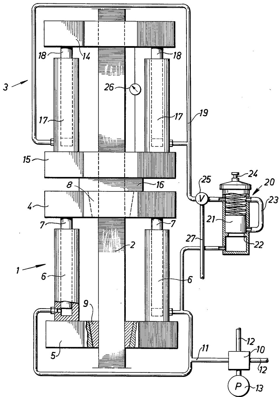
**APPARATUS FOR OBTAINING SUBSTANTIALLY EQUAL STEPLENGTH OF EACH JACK IN A GROUP OF PRESSURE FLUID OPERATED CLIMBING JACKS**
