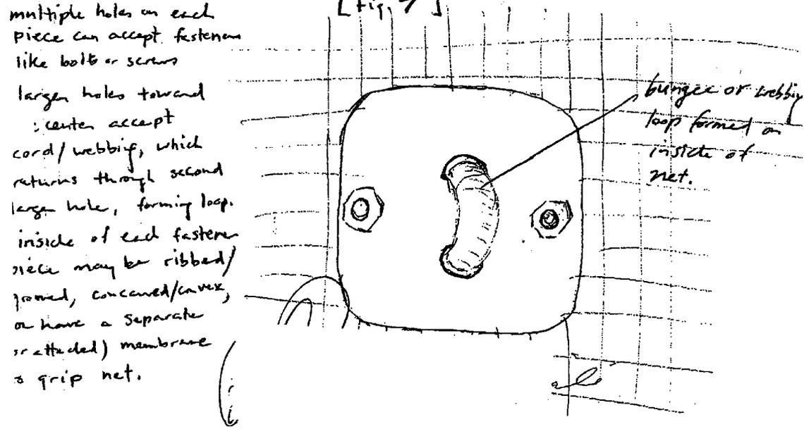
[Figure 8] View of fastener from inside of enclosure w/ webbing installed
