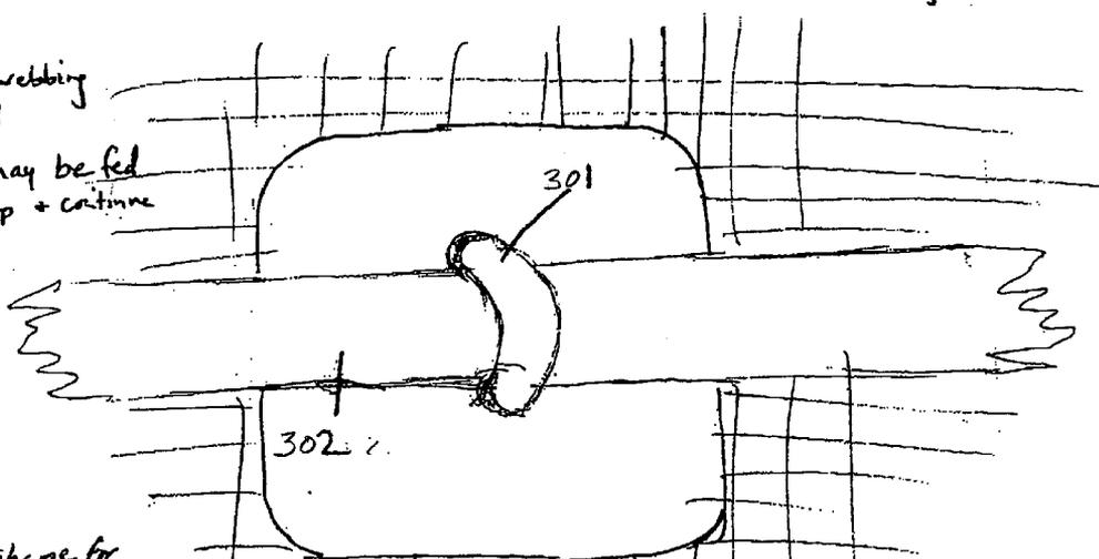
3) possible shape for membrane acting as impact absorber
