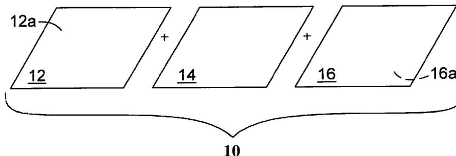
(57) Abstract: A solar collector with reflective composite sheets consisting of a solid thermoplastic core between an outer aluminum skin. The reflective sheets are secured together with stiffeners formed from the same reflective composite sheet material. The sheets may be connected in modules for securing to longitudinal supports to establish the solar energy reflective surface of the solar collector.
