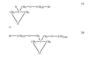
The repeat unit of a polyfluorooxetane polymer derived from the oxetane monomer 1A or 1B with a monoalcohol initiator respectively has the formula
