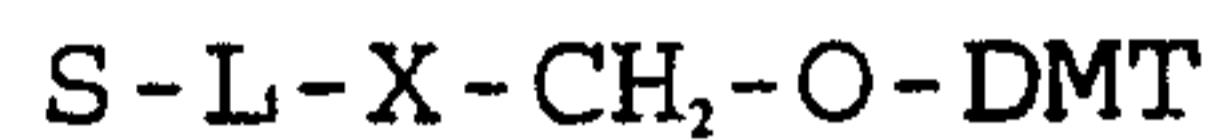
wherein S is a solid support material, L is a linker group, said linker group being cleavable by appropriate means at the end of oligonucleotide synthesis to release the completed oligonucleotide product, X contains either a polymerizable ethylene-containing monomer unit or a chemically protected version of same, which can be deprotected using appropriate techniques, and DMT is a 4,4'-dimethoxytrityl group.
