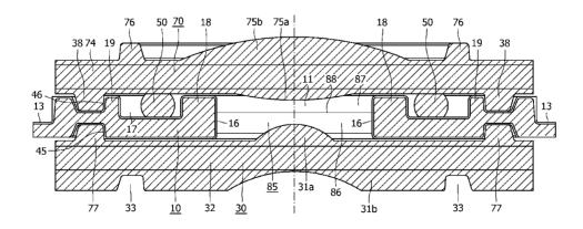
(57) Abstract: The electrowetting optical element comprises a first electrically conducting fluid and a second electrically insulating fluid. According to the invention the second fluid comprises a compound including an aliphatic ring-structure. The optical element may be a lens or a zoomlens or be part of a zoomlens system.
