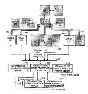
(57) Abstract: A computing system is described that includes an I/O unit interface that is deactivated while said computing system operates within a non main CPU/OS based operational state. The computing system also includes a controller that operates functional tasks while the computing system is within the non main CPU/OS based operational state. The computing system also includes an I/O unit that is coupled to both the I/O unit interface and the controller.
