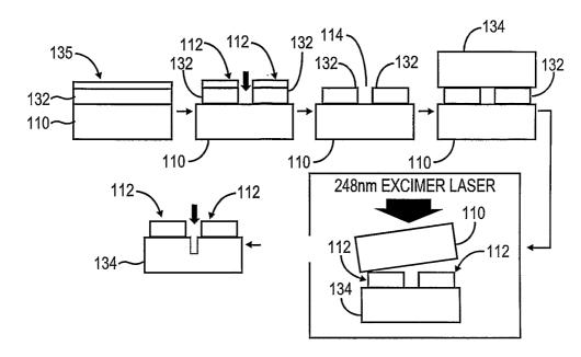
(57) Abstract: A lift off process is used to separate a layer of material from a substrate (110) by irradiating an interface between the layer of material and the substrate (110). According to one exemplary process, the layer is separated into a plurality of sections (112) corresponding to dies on the substrate (110) and a homogeneous beam spot is shaped to cover an integer number of the sections (112).
