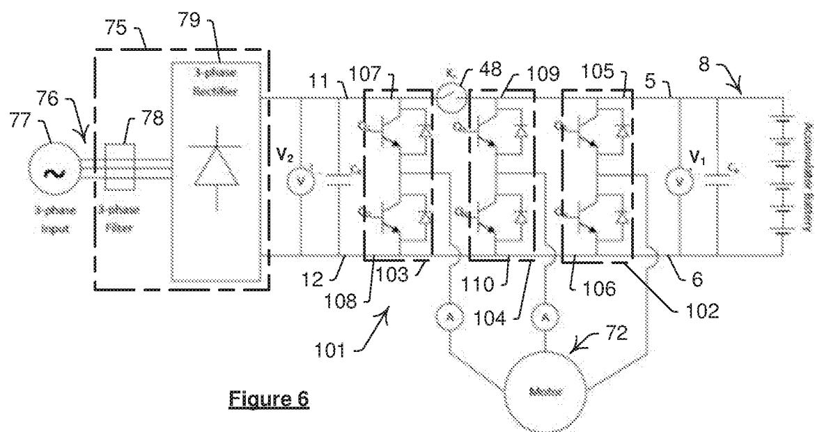
Buck Mode -  $V_2 > V_1$
