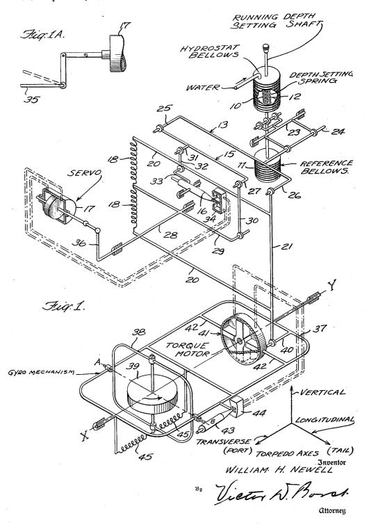
DEPTH CONTROL MECHANISM FOR DIRIGIBLE SUBMARINE
