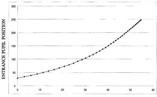
AMOUNT OF MOVEMENT OF SECOND LENS GROUP IN OPTICAL AXIS DIRECTION
