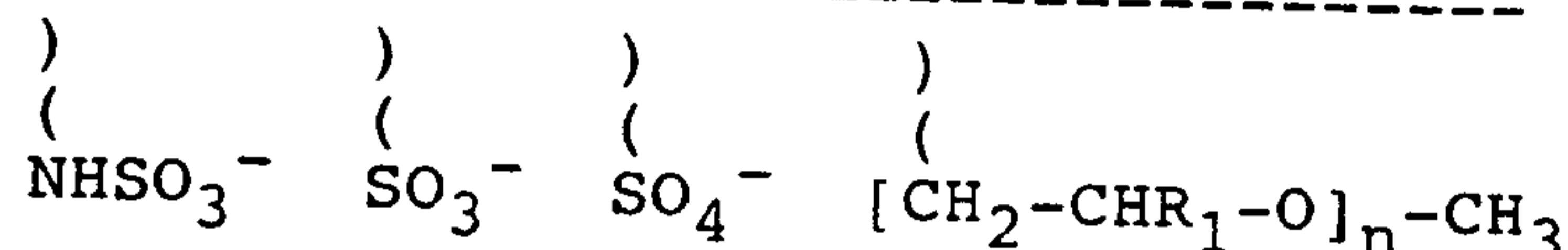
The above co-polymerised monomer compositions are examples of non-thrombogenic (NON-TH) polymers represented above as Type 1.
