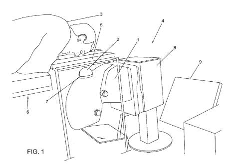
(57) Abstract: Apparatus (1) for creating an optical coherence tomography image of the back of an eye, wherein a light beam operatively exiting from the apparatus has a main axis. The main axis of the exiting light beam has a substantially standing orientation. At least an exit unit of the apparatus is height adjustable along the main axis.
