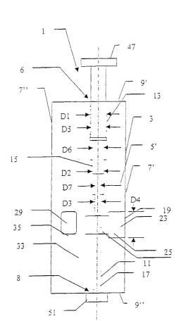
(57) Abstract: A loader device, for dispensing implantation seeds from a seed magazine, comprising a body (3), seed magazine receiving and locating means (27), seed dispensing means (37) for ejecting seeds from a seed magazine, and a seed-transporting path (17) leading to a dispensing outlet (8), which loader device further comprises a spacer-transporting path (29, 31, 33, 35) for transporting spacers through the device to the dispensing outlet (8).
