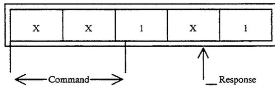
With respect to the above command sequence, it is important to note that with respect to any transponders 10 which may enter the powering RF field late, that only by specifically sending the RESET0 command from the powering controller 12 is there the possibility of any transponder 10 receiving two zero's in a row and thereby interpreting the same as the RESET0 command ("00").
