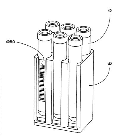
(57) Abstract: Automatically entering data (40BC) into a clinical analyzer's (10) operating control system, the data (40BC) associated with an object (40, 42) to be placed into the clinical analyzer (10), by providing special symbols (40BC) as an additional identifier in indicia (40BC) affixed to the object (40, 42).
