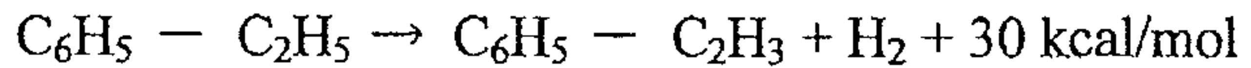
The dehydrogenation reaction was studied intensively in the 1940s in the U.S.A. to meet the social demands for the production of synthetic rubber. During the period, a system of dehydrogenating ethylbenzene with contact under steam dilution was established technically, which is now employed globally and it has become a typical method for production of styrene.
