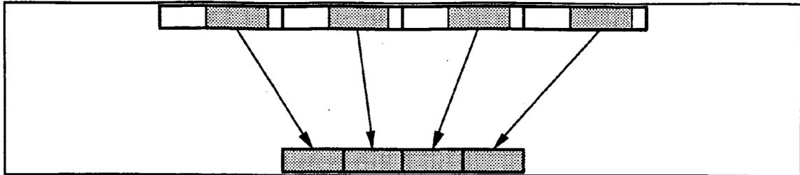
**Compress 32 bits to 16, with 4-bit right shift**
