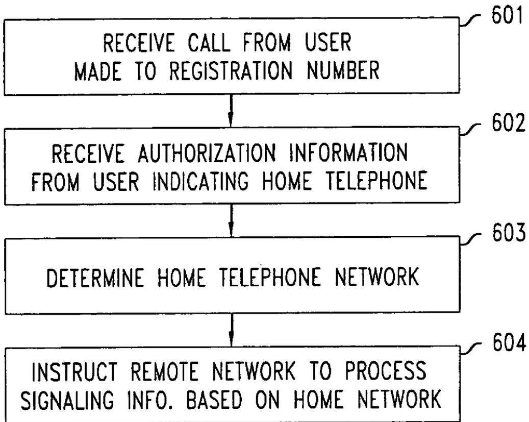
**"ROAMING" METHOD AND APPARATUS FOR
