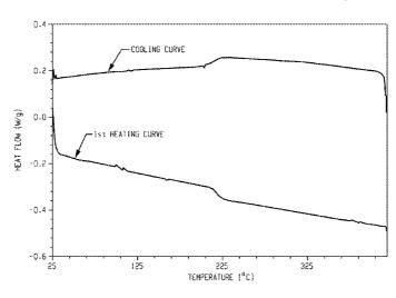
talline polyphenylsulfone, which exhibits a crystalline melting point in a range of 215 to 270° C., can be prepared from amorphous polyphenylsulfone using a solvent-induced crystallization method. An additive manufacturing method utilizing particles of the semicrystalline polyphenylsulfone is described.
