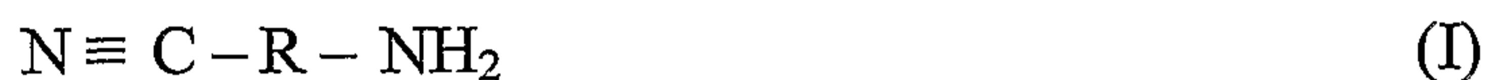
15 in which R is an alkylene group having 3 to 12 carbon atoms. The preferred compound of formula (I) is 6-aminocapronitrile (ACN), which produces ε-caprolactam (CPL), the polymerization of which leads to the synthesis of Nylon-6.
