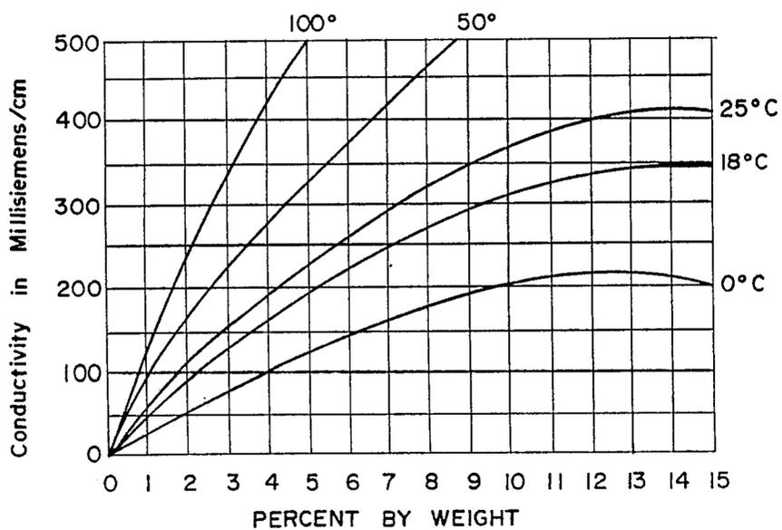
Conductivity versus Concentration for Sodium Hydroxide (NaOH)
